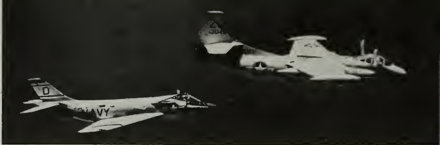
TEAMWORK—Prop-driven AJ re-gases fuel-consuming jet while in flight.
